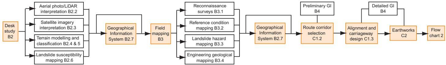
**Flow chart 2: Design and construction of new slopes (for new road construction and road improvement)**
